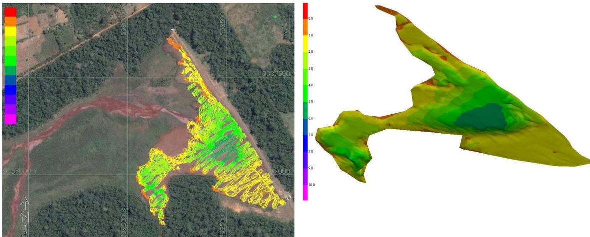
**Figure 06: Bathymetric data and 3D graphic of the dam Geladinho in July 2008**
