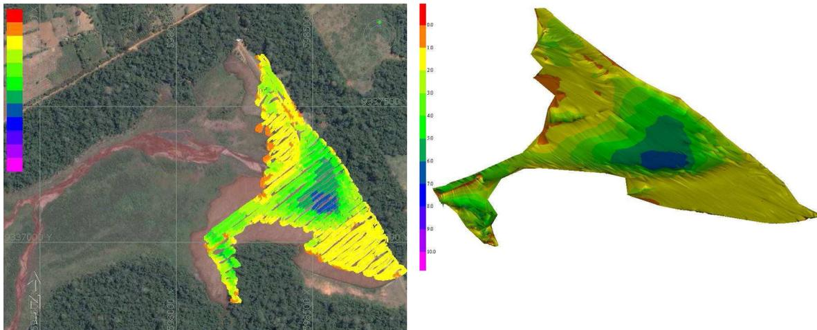
**Figure 05: Bathymetric data and 3D graphic of the dam Geladinho in April 2008**
