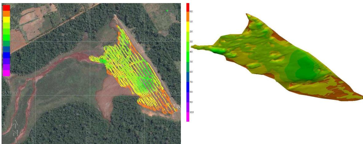
**Figure 07: Bathymetric data and 3D graphic of the dam Geladinho in October 2009**
