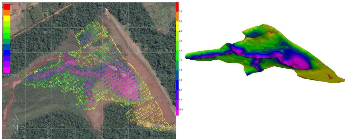
**Figure 03: Bathymetric data and 3D graphic of the dam Geladinho in November 1999**
