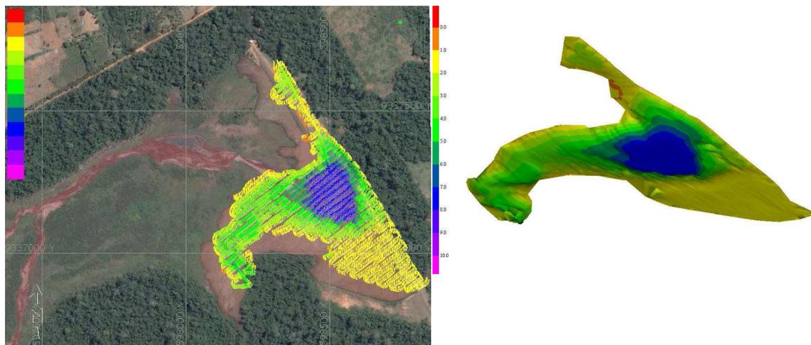
**Figure 04: Bathymetric data and 3D graphic of the dam Geladinho in December 2005**
